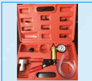
No,014(1) Leaking Testing Tools For Valve Assembly
