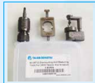
NO,087(3)Dismounting And Mesuring Tools For CRIN1 Spacer And Armature
